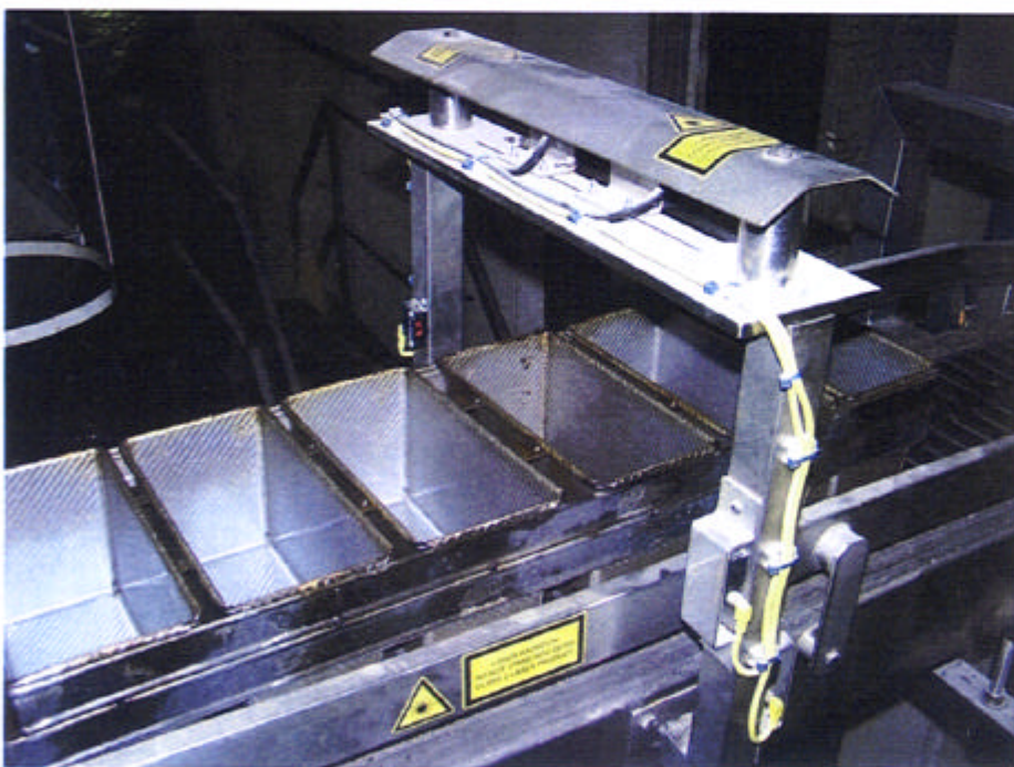
C F Controls' Carbonised dough system detects foreign bodies and items not detected by other systems
